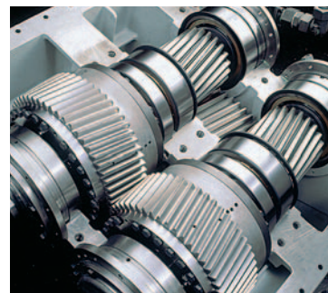
Rolling mill gearbox with tapered roller bearings and cylindrical roller bearings
