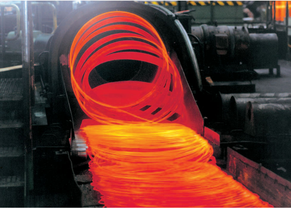
High-speed laying head with special cylindrical roller bearings, angular contact ball bearings, and spindle bearings
